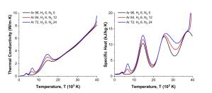
Fig. 1. Thermal conductivity and Specific heat for gas mixture
